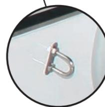
Internal & external towing/ lifting points
